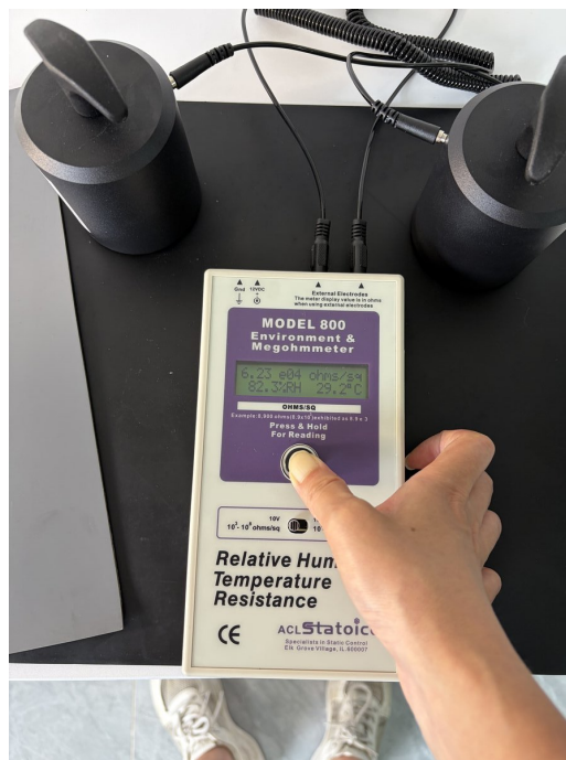
PTP-B04 — black conductive layer, 6.23 \times 10^4 ohm at 82.3 %RH, 29.2 °C.
