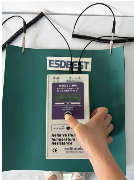
PTP-T02 — green dissipative layer, 2.01 \times 10^6 ohm at 81.7 %RH, 29.4 °C.
