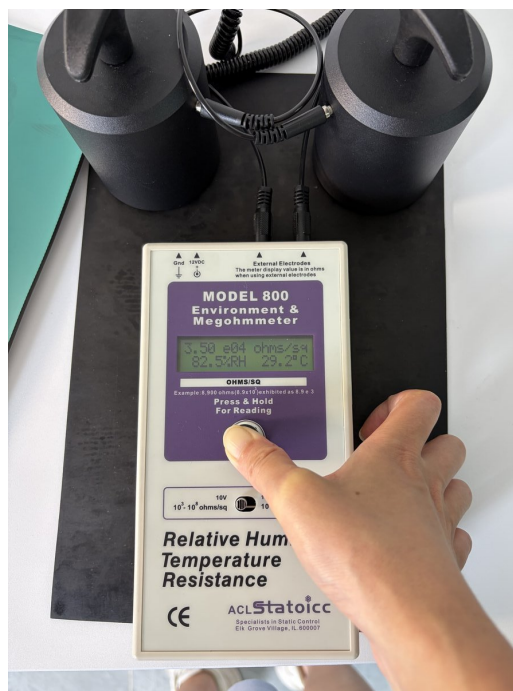
PTP-B06 — black conductive layer, 3.50 \times 10^4 ohm at 82.5 %RH, 29.2 °C.
