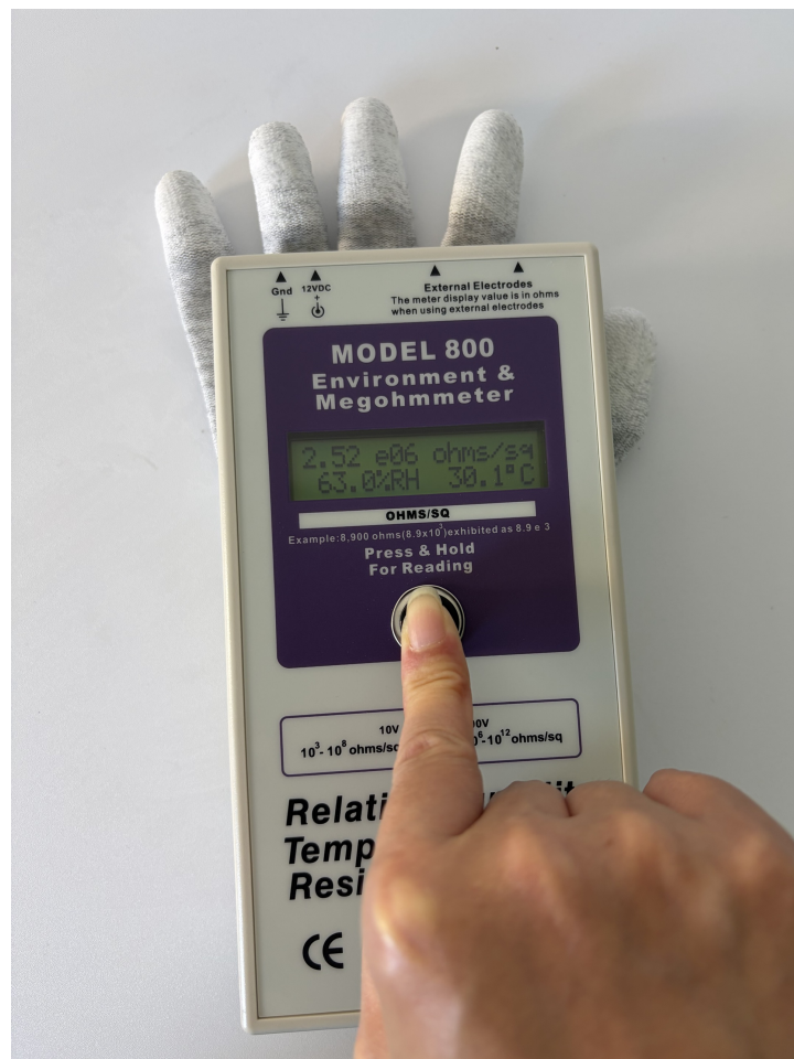
Figure 2 — Sample A, reading A-01: 2.52 e06 ohms/sq at 63.0% RH, 30.1 °C.
