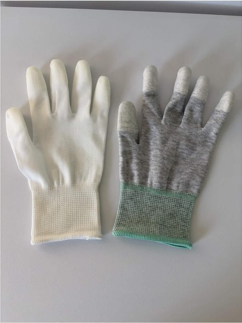
Figure 1 — Sample C (left, plain knitted) and Sample A (right, carbon fibre). Same knit, same PU fingertip coating.
